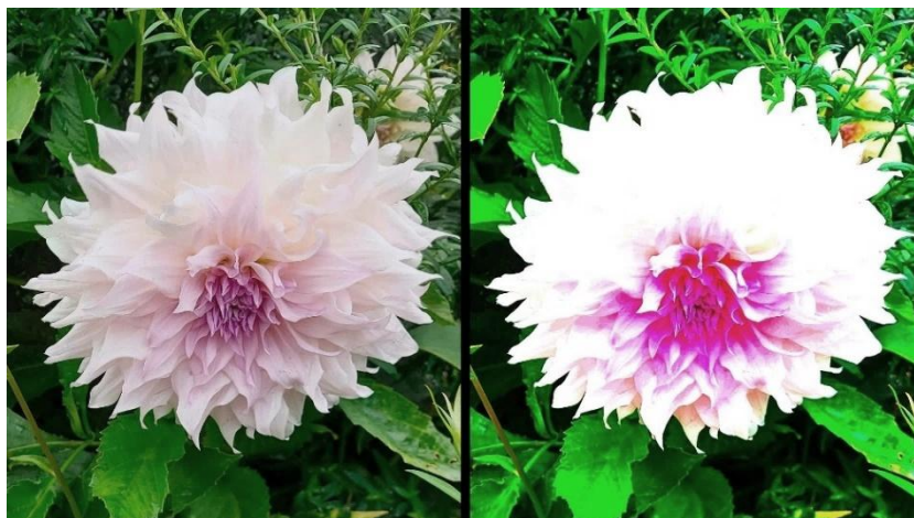
Figure 8: Non-conversion from SDR (left) to HDR10 (right) leading to burned colors
