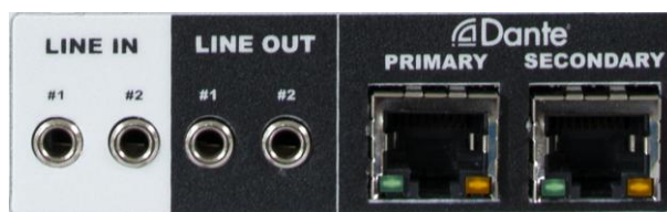
Fig. 4 - Analog and Dante audio card
